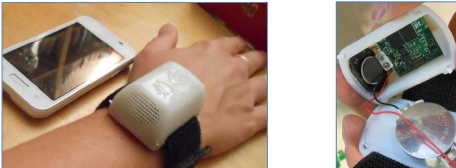
Figure 2. ABBI device and ABBI battery and micro-speaker
