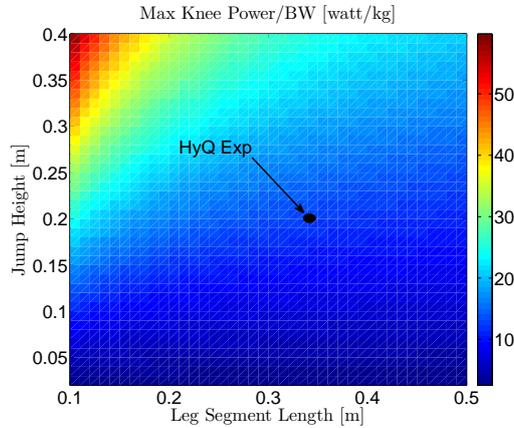
Fig. 4. Plot of maximum knee joint power scaled by body weight BW for different leg segment lengths and jump heights. The arrow marked with *HyQ Exp* shows the experimental results obtained with HyQ as an example.
