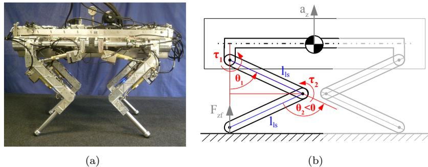
Fig. 1. HyQ: Hydraulic Quadruped robot. (a) picture and (b) sketch of side view of robot in squat posture, defining the centre of mass (COM) acceleration vector  $a_z$ ; joint angles  $\theta_{1,2}$  and torques  $\tau_{1,2}$  of the hip and knee joint, respectively; leg segment lengths  $l_{ls}$  and ground reaction force vector at the foot  $F_{zf}$ .
