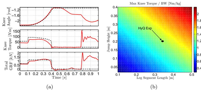
Fig. 2. **(a)** Plot of experimental data (red solid) and simulated data (black dashed) for a squat jump motion of 0.2m jump height. *Top*: knee joint angle  $\theta_2$ ; *middle*: knee torque  $\tau_2$ ; *bottom*: total ground reaction force  $4F_{zf}$ . **(b)** plot of maximum knee joint torque scaled by the robot's body weight (BW) for different leg segment lengths and jump heights. The arrow marked with *HyQ Exp* shows the experimental results obtained with HyQ as an example.
