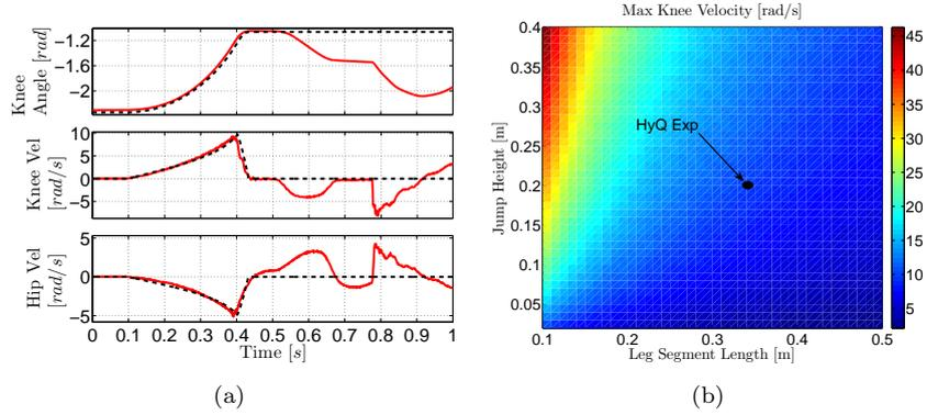
Fig. 3. (a) Plot of experimental data (red solid) and simulated data (black dashed) for a squat jump motion of  $0.2m$  jump height. *Top*: knee joint angle  $\theta_2$ ; *middle*: knee joint velocity  $\dot{\theta}_2$ ; *bottom*: hip joint velocity  $\dot{\theta}_1$ . (b) plot of maximum knee joint velocity for different leg segment lengths and jump heights. The arrow marked with *HyQ Exp* shows the experimental results obtained with HyQ as an example.
