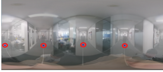
Fig. 2: Equirectangular image transformed from an omnidirectional capture and points (blue dots inside red circles) representing calibrated threshold line ( 3 \pm 0.1 m from the wheelchair) which utilized to detect the danger zone.
