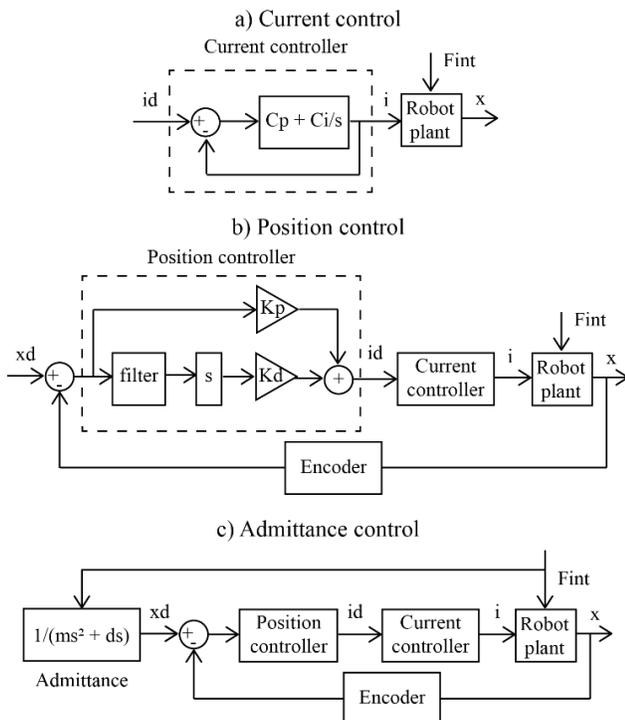
Fig. 2: Control diagrams for a) current control:  $i_d$  = desired current,  $i$  = actual current,  $C_p$  = proportional gain,  $C_i$  = integral gain,  $F_{int}$  = interaction force,  $x$  = actual position, b) position control:  $x_d$  = desired position,  $K_p$  = proportional gain,  $K_d$  = derivative gain, and c) admittance control:  $m$  = virtual mass and  $d$  = virtual damping.
