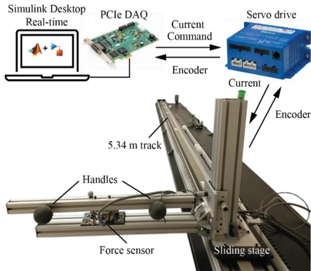
Fig. 1: Robotic emulator components and communication pathways
