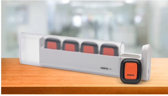
Fig. 1. XSens DOT charging case and 5 IMUs.
