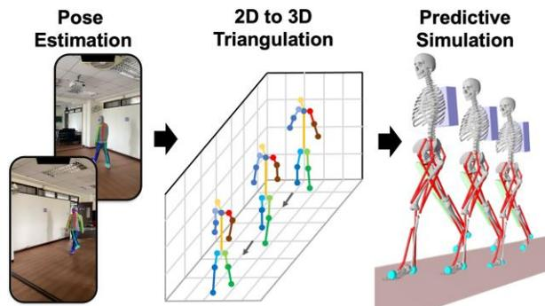
**Figure 1.** Schematic of the musculoskeletal model derived from the 2D pose estimations then adding exoskeleton assistance. The potential distortion of the model was analyzed by adding ground inclination and backpack loads to investigate the effect of muscle strength and walking gait adaptation.
