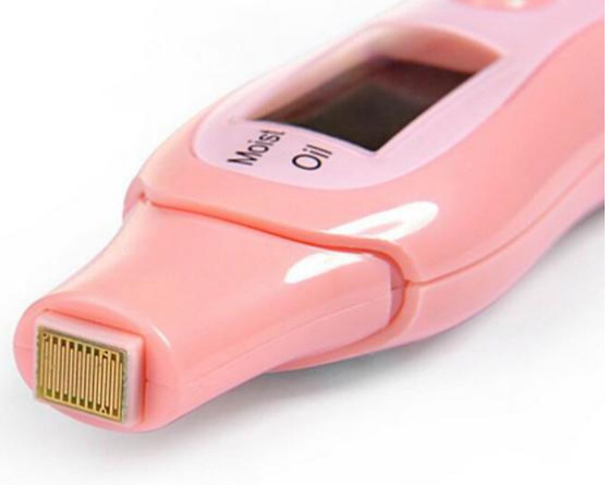
Figure 12. The electrical circuit is visible on the top of the sensitive head. (Neon SK-5D, commonly sold on Amazon)
