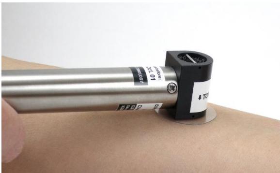
Figure 13. The chamber of the TEWL sensor.
