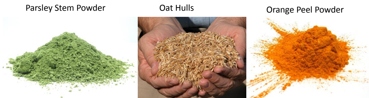
Figure 7. Examples of agro-waste raw materials that can be used to produce bioplastics
