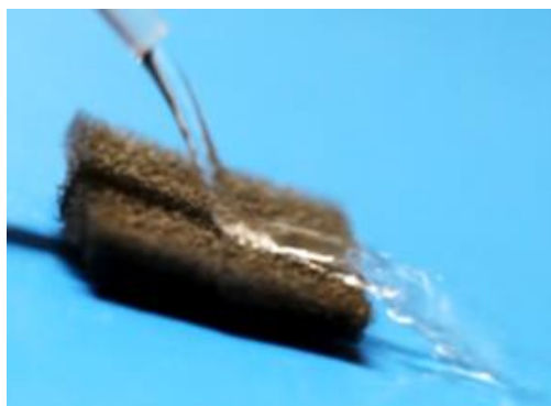
Figure 4. A jet of water repelled by the functionalized polyurethane foam due to its treatment by superhydrophobic particles
