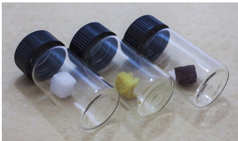
Figure 7. Elastomeric foam before (white), after ZnSe treatment (yellow), and after removal of Pb^{2+} ions from water (dark brown)
