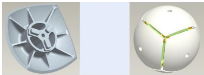
An Instrumented sphere. Attaching the spherical faces an instrumented sphere is created.
