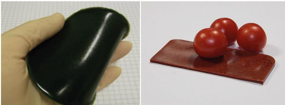
**Figure 6.** Bioelastomers obtained from spinach and from tomato skin residue originating from tomato pulp making
