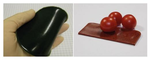
Figure 6. Bioelastomers obtained from spinach and from tomato skin residue originating from tomato pulp making
