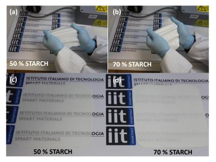
**Figure 4.** Photographs of bio-elastomers containing (a) 50% and (b) 70% unmodified corn starch granules. Photographs in (c) and (d) show that the bio-elastomers are somewhat transparent when placed on a surface, macroscopically indicating good degree of starch particle dispersion
