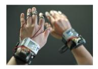
For example, Finger-Braille interfaces with wristwatch computers have been developed and are capable to send information to the blind person. The computers are linked to six fingers (three per hand), which receive vibrations according to Braille language. This system allows to interact through Bluetooth devices.
