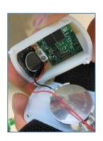
Figure 2. ABBI device and ABBI battery and micro-speaker
