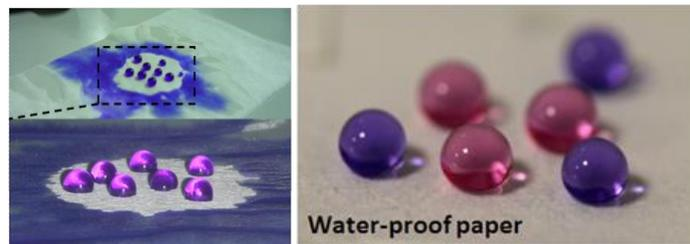
**Figure 4.** Hydrophobic properties: dyed water cannot enter the treated central area of the paper
