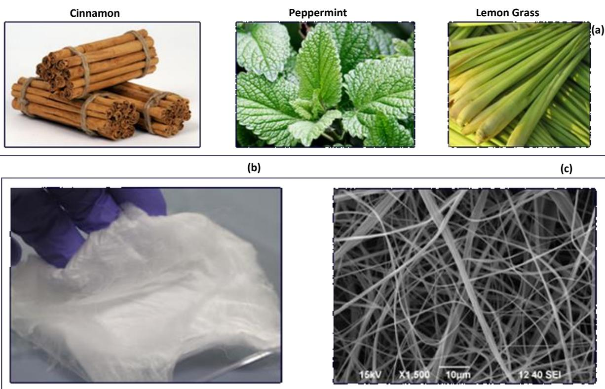
**Figure 10.** (a) Photograph of the plants used for the extraction of the essential oils. (b) Photograph of the produced electrospun mat and (c) corresponding SEM image.
