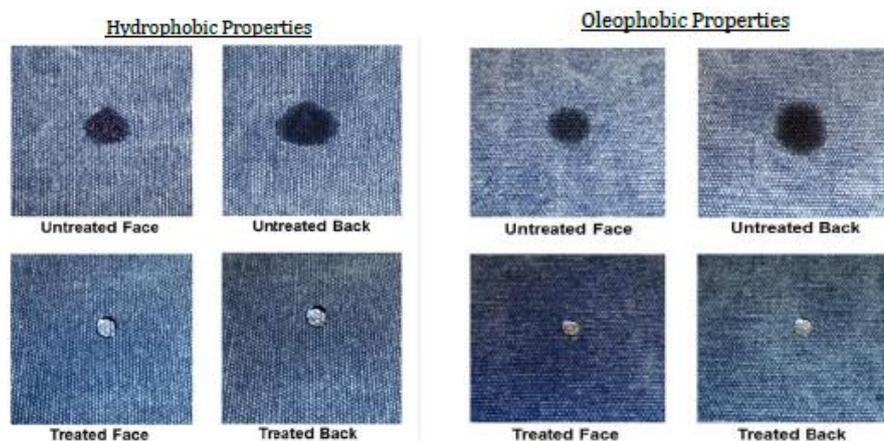
**Figure 6.** Images of a water (left) and oil (right) droplet on a cotton textile before and after treatment
