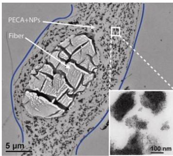
**Figure 3.** Cross section of a single cellulose fiber with the polymeric composite material cladding around it (electronic microscope)
