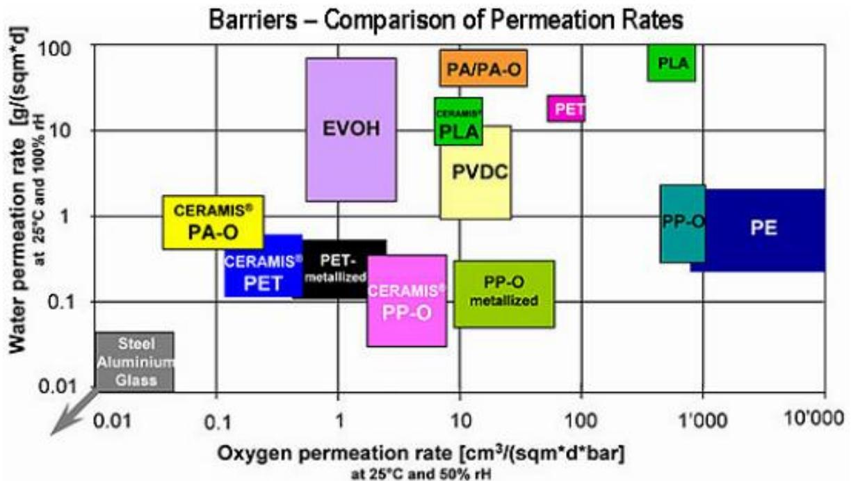
Figure 16. Oxygen and water permeation rates for various types of barrier films
