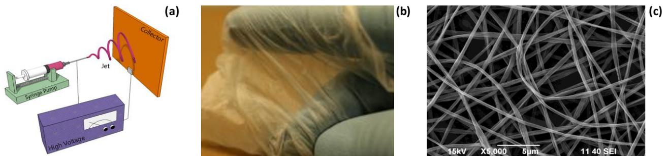
**Figure 8:** (a) Electrospinning apparatus consisting of a syringe pump for the delivery of the polymer solution and a plate for the collection of the fibres. The high voltage is applied between the metallic needle and the collector. (b) Photograph of an electrospun mat and (c) corresponding scanning electron microscope (SEM) image.
