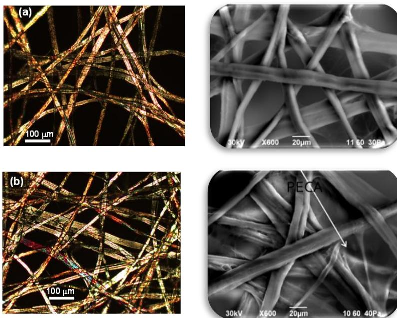
**Figure 2.** Optical and electronic microscope images of (a) untreated and (b) treated cellulose fiber networks with acrylate-based polymer (fibers are clearly visible in both cases and the breathability is conserved after the treatment)
