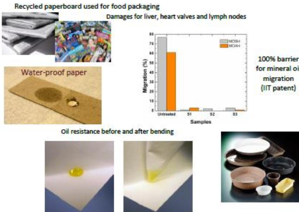
**Figure 7.** Polymeric composite nanomaterial as a barrier to mineral oil migration
