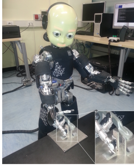
FIGURE 2.6: The setup used to characterize the tactile response for hard objects.
