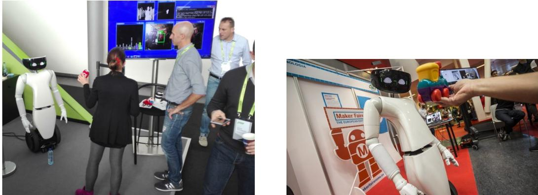
Figure 1.2: **Snapshots from the ON THE FLY RECOGNITION demo** developed within the Thesis. The robot is able to quickly learn the appearance of novel objects through a natural interaction with humans, recognizing them reliably in unconstrained environments. Details on the demo are provided in Chapter 9; (Left) GPU Technology Conference, Amsterdam; (Right) Maiker Faire, Rome.
