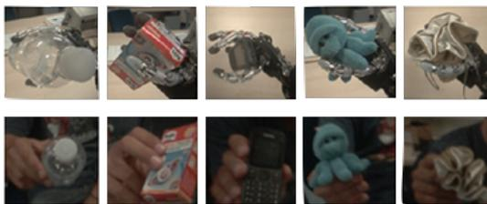
Figure 5.2: Example images showing objects acquired in Human and Robot modes.
