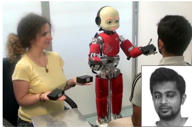
Figure 21. HRI study setup: the robot is offering a building block to the subject with its left hand. Lower right: gaze estimation by iCub on the subject before the offering action.
