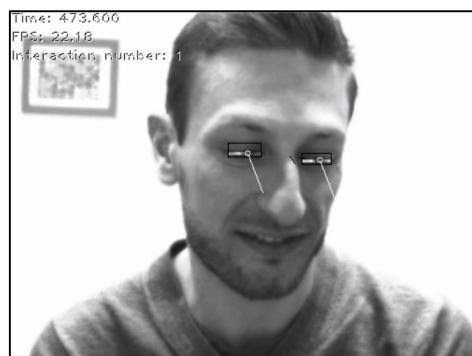
Figure 24. Example output of our eye tracking system. White lines from eyes – eye gaze, black line from top of the nose – head gaze.
