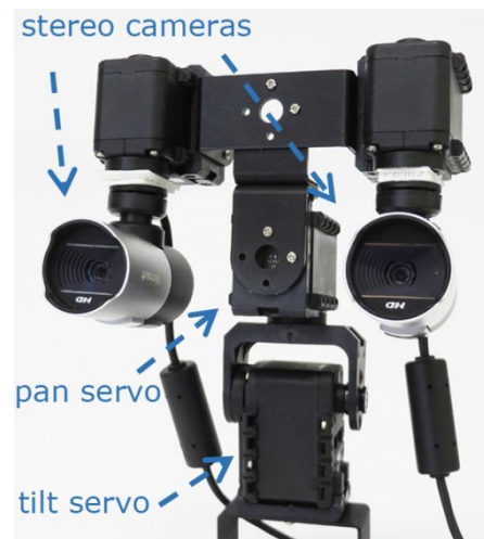
Figure 6. Camera and motor setup.
