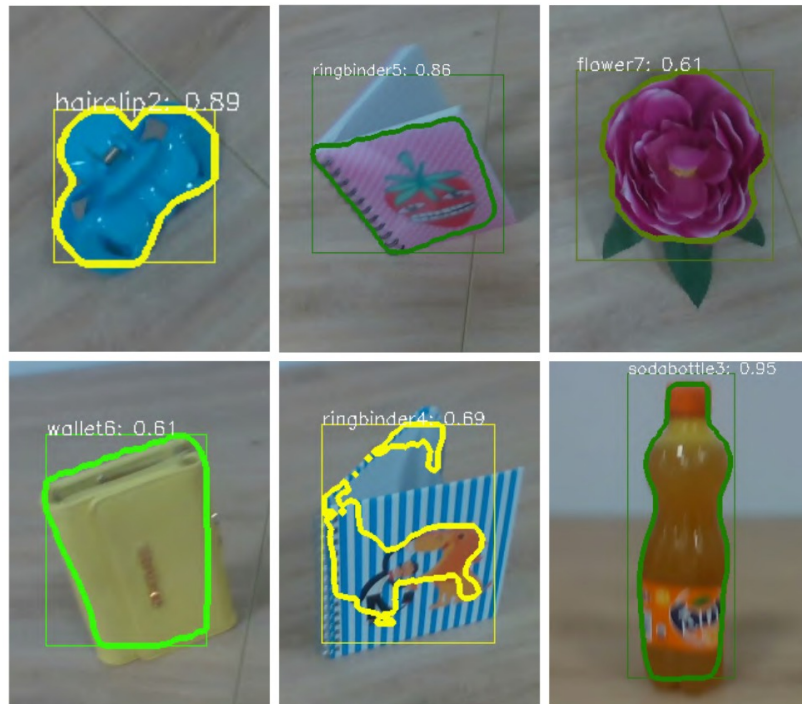
Figure 7.7: This picture is taken from Bunz (2019) and it shows randomly sampled examples of bounding boxes and segmentation predicted by the proposed pipeline.
