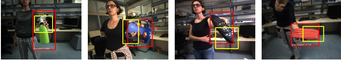
Figure 6.2: Example frames where the trained detector (either ZF or VGG_CNN_M_1024) outputs a correct bounding box around the object (red), while the depth segmentation fails (yellow).
