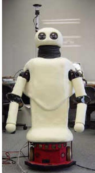
**Figure 2.12:** The humanoid robot Robovie-IIS (Tajika T. and H. (2006)).
