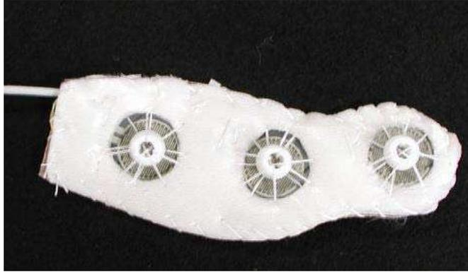
**Figure 2.6:** Placement of the pressure transducers in the Robonaut hand (T. B. Martin and J. Butzer (2004)).
