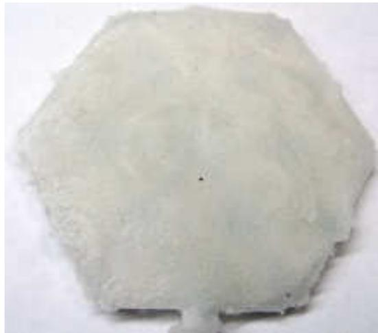
**Figure 6.10:** After the placing of the board the mold is poured with silicone rubber foam
