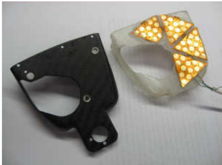
**Figure 6.15:** The triangles are glued on the fiberglass mold.
