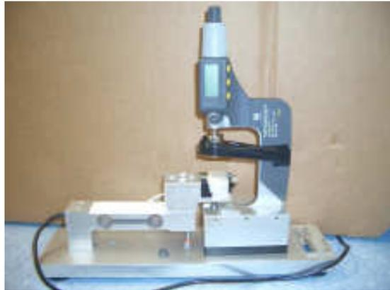
**Figure 7.1:** Test setup with a load cell that can measure static forces. The off-center load cell (3 kg AL series, from Laumas) and the micrometer (TESA Micromaster IP54) are shown
