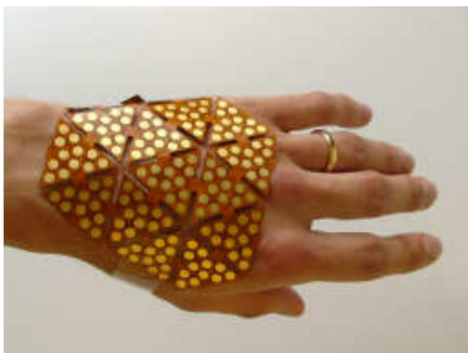
**Figure 1.1:** The tactile sensor PCB rests on a human hand
