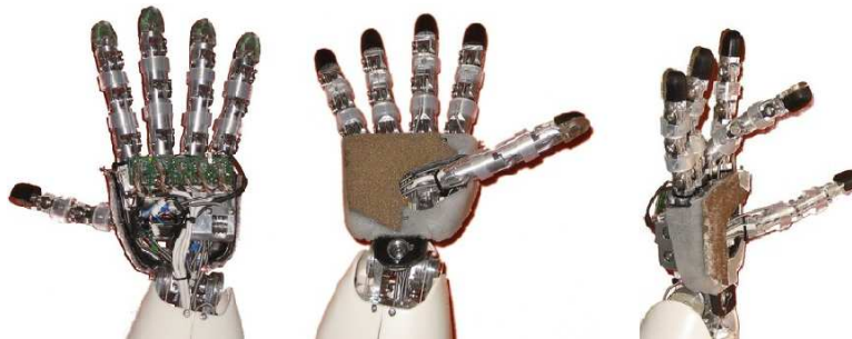
Figure 2.6: The iCub hand: in evidence, the embedded electronics (a MAIS board on the top), the tactile skin covering the palm and the tactile fingertips. More details can be found in [Schmitz et al., 2010].
