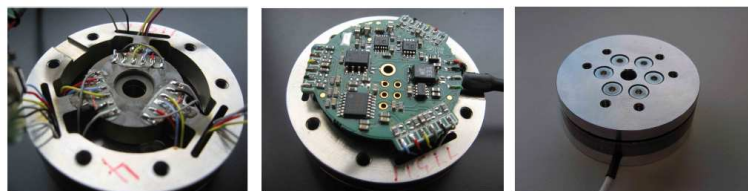
Figure 2.8: The custom FTS developed for iCub. Left: the sensing element. Center: the embedded electronics. Right: the assembled sensor. Notice the CAN line, going out from the sensor, which transmit sampled digital measures at 1ms rate (image from [Fumagalli et al., 2010b]).
