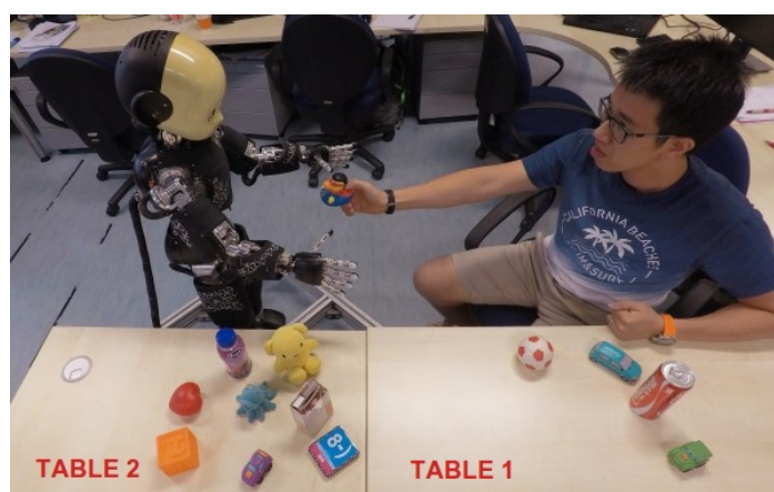
Figure 2.12 The Human Robot Collaboration (HRC) experimental setup for [78]. The human is sitting next to Table 1 while the iCub is located near Table 2 , effectively sharing the workspace.
