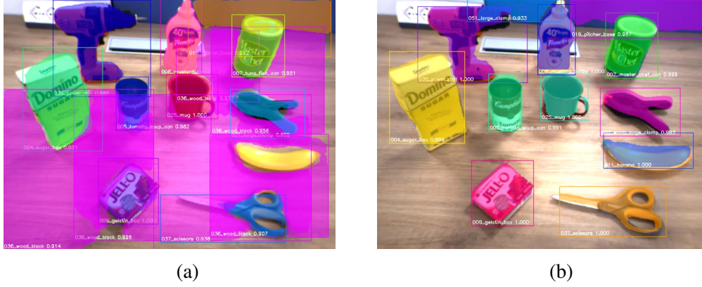
Figure 3.5 Samples of instance segmentation output from a real scene using a Mask R-CNN model trained with our approach. In (a), the purple regions correspond to false detections of the wood_block object. (b) shows the output of the network when trained on a similar dataset that does not include the YCB wood_block object.
