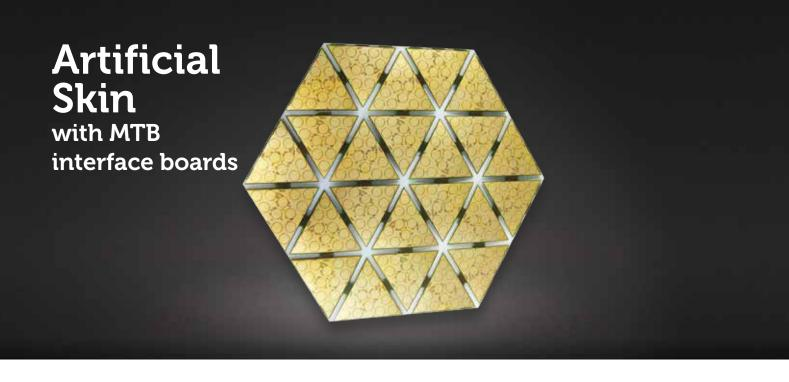
Large Area tactile sensor based on capacitive technology. Up to 16 triangles with 12 sensors each (192 taxels) interconnected on a flexible-pcb driven by a microcontroller board (MTB). The skin can be cut from the triangular panel and applied to any 3D surface.
