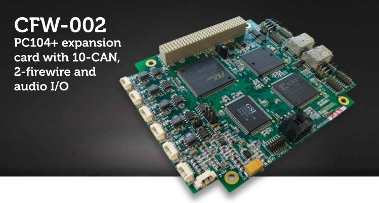
The CFW-002 board is PC104+ standard expansion card directly connected to the PC104+ bus. The board has 10 CAN Bus 2.0B links, 2 IEEE 1394 (Firewire) high speed ports, one stereo microphone preamplifier and a single D-Class speaker output.
