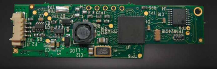
The **MAIS** is a miniature board for the acquisition of 15 analog signals that can be used to interface absolute position sensors in hall effect or resistive technology.
