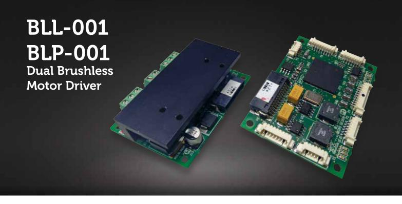
This motor controller is made of two separate boards. The BLL contains the logic circuits, while the BLP includes the power drivers. The controller is capable of driving up to two 250W Brushless DC motors using CAN bus communication for command and control data exchange.
