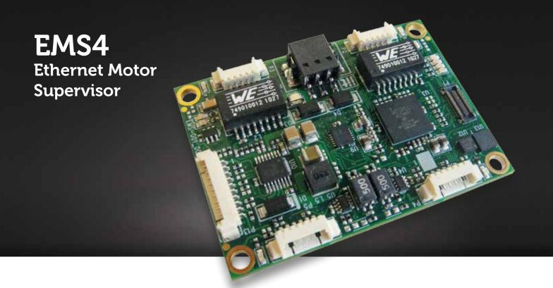
The EMS4 card is a 32-bit Arm Cortex-M4 embedded microcontroller based device designed for managing several communication channels in robotic applications. Its main function is to provide the bridges among two Ethernet 10/100 base-T high-speed link, two CAN-2.0B buses and six SPI-master buses. When connected to external motor-driver cards (i.e. 2FOC, BLL/BLP or MCP/MC4), the EMS4 embedded microcontroller provides enough computational power to directly manage up to four motor control-loops.
