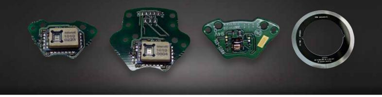
The Reflective Optical Encoder in two different sizes (ROIE, ROIEL) and LCORE (Low Cost Reflective Encoder) boards are a series of incremental encoders with resolution from 1000 to 4000ppr (4000 to 16000cpr). The encoders use low cost reflective disks or linear scales.
