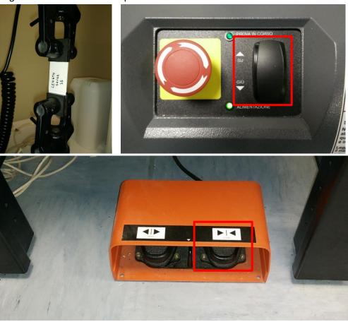
b. Click on Zero Displacement. The Displacement signal should now be 0
