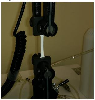
f. If you are using the SVE, be sure that the sample is visible in the SVE frame and that the dots are properly grabbed by the software (red frame boxes). The detection area, indicated by a green box, can be modified by dragging the finger or mouse pointer over the desired zone.
