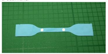
d. Tension only: mount sample inserting one end on the top clamp and close by pressing once the CLOSE pedal
