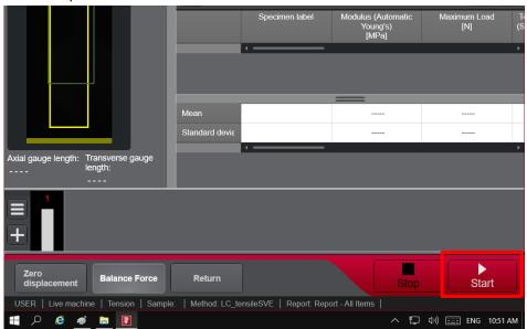
h. The standard method is set to detect sample failure. However, the algorithm does not always successfully detects the break. When the sample breaks and the machine does not stop, click or tap on the *Stop* button. Then remove the sample by pressing the OPEN pedal and click or tap on the *Return* button. The clamp will return to the starting position (*displacement=0*)
