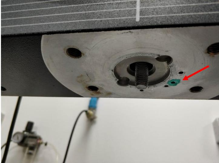
8. Tighten the top screw with the 8 mm hex key
