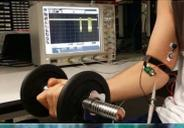
Spike-level EMG signals TX mini-module comprising integrated amplifier, interface and IR-UWB transmitter (Average Threshold Crossing)
