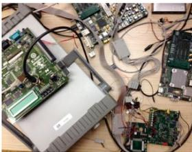
FPGA testbed for the protocol test (PC interfacing and error-rate validation)
