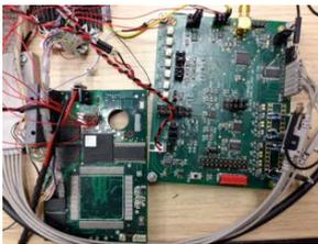
Quasi-digital read-out circuit IC (tactile sensing) connected to iHead
