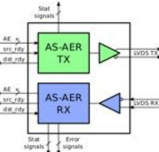
Block scheme of the AS-AER integrated interface
