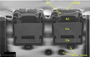
Gold plated CMOS micro-electrodes (on-chip post-processing)
