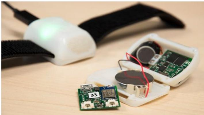
**Problem solved:** Fit a full 9 DOF IMU system with sophisticated audio and radio communication capabilities in a device small enough to be wore by babies.
