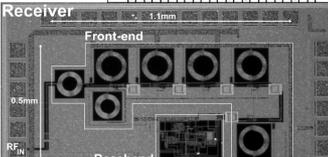
Interference Robust 130nm IR-UWB receiver for analog/digital-mode Wireless links
